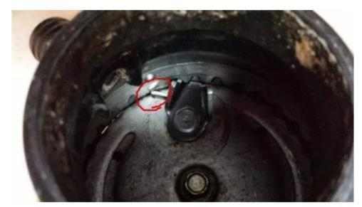
The flywheel on this garbage disposal is jammed by a piece of metal that fell into the drain. Although food is often the culprit of a jam, other items and debris like this metal piece can accidentally cause failure.
