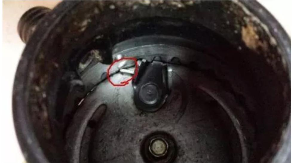
The flywheel on this garbage disposal is jammed by a piece of metal that fell into the drain. Although food is often the culprit of a jam, other items and debris like this metal piece can accidentally cause failure.
